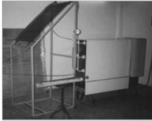
Fig. 16. Heat pump with three adsorbers and a condenser/evaporator, intended for use in a system of energy trigeneration (production of electricity, heat, and cold) and operating with two pairs of adsorbers in antiphase.
